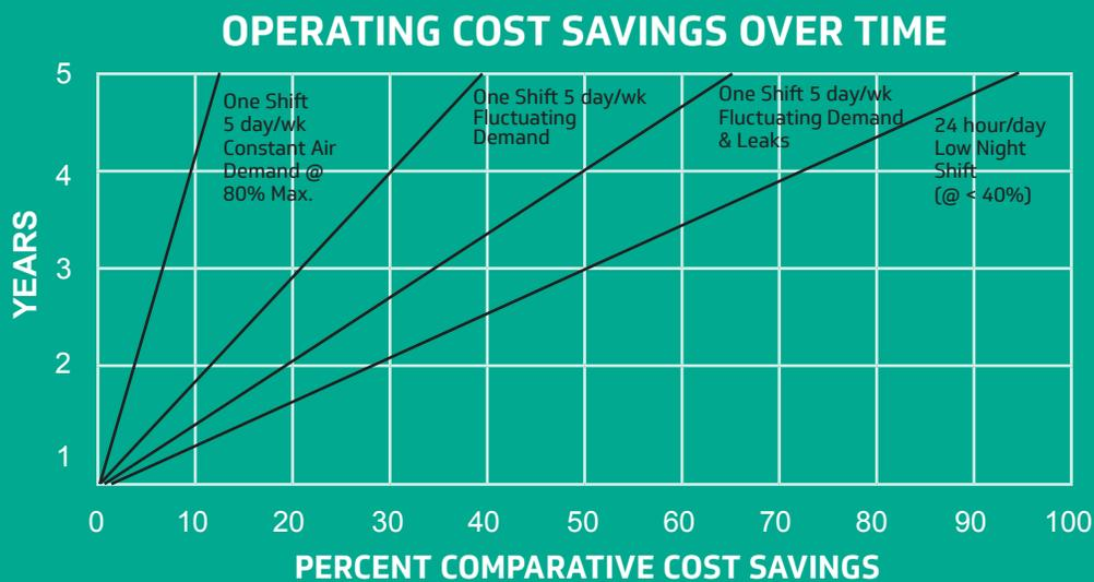
The Cost Savings Chart illustrates the reduced operating cost of a VFD Unit by correcting poor air usage: Five day/week operation, erratic demand fluctuations (28% of installations), steady weekend consumption with leaks (64% of installations). This shows 24 hour operation with low night shift and high day shift consumption at more than 40% savings after 5 years. **In many instances the VFD Compressor will have a payback of the additional cost within 2 1/2 to 3 years.**
