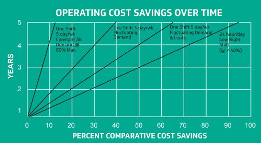
The Cost Savings Chart illustrates the reduced operating cost of a VFD Unit by correcting poor air usage: Five day/week operation, erratic demand fluctuations (28% of installations), steady weekend consumption with leaks (64% of installations). This shows 24 hour operation with low night shift and high day shift consumption at more than 40% savings after 5 years. In many instances the VFD Compressor will have a payback of the additional cost within 2 1/2 to 3 years.
